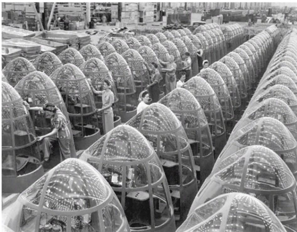
Fig 4.3 Female workers and the nose sections of A-20 bombers at the Douglas plant in Long Beach, California, October 1942. Alfred Palmer (Office of War Information), NARA file #208-AA-352QQ-5.
