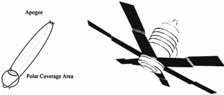
Figure 3.6: Molniya satellite and orbit
