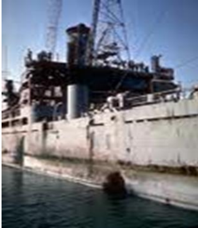
Fig. 10, Torpedo hole in starboard side of ship.
