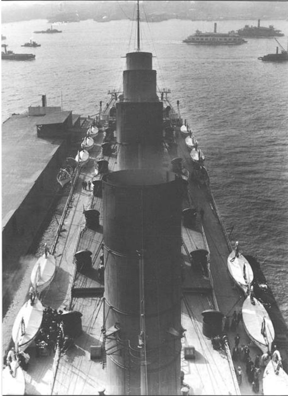
View towards the Lusitania 's stern, showing her four tall funnels and her lifeboats hanging from their davits.
