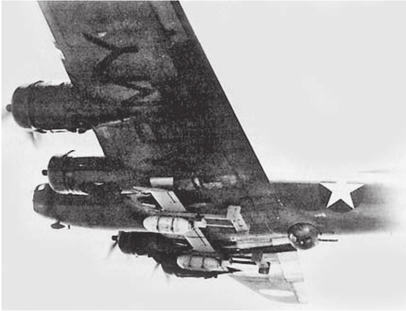
Two GB-1 glide bombs slung under a B-17 for testing. The results of experimental attacks on Cologne with these munitions in 1944 were disappointing, and the GB-1s were never used in combat again.
