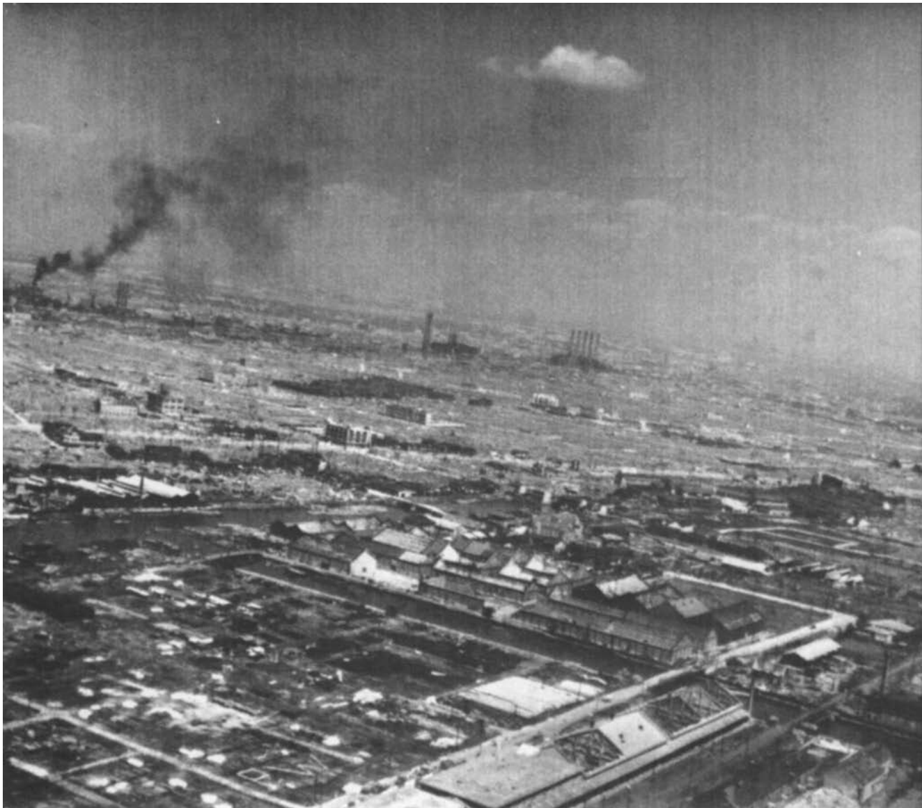
photograph (22) taken in September 1945 testified to the destruction of an unidentified Japanese city on Honshu, with a partially demolished POW camp in the foreground. Some structures appear intact in these photographs, but appearances could be misleading: the walls of concrete buildings often survived incendiary attack, but fire gutted them.
