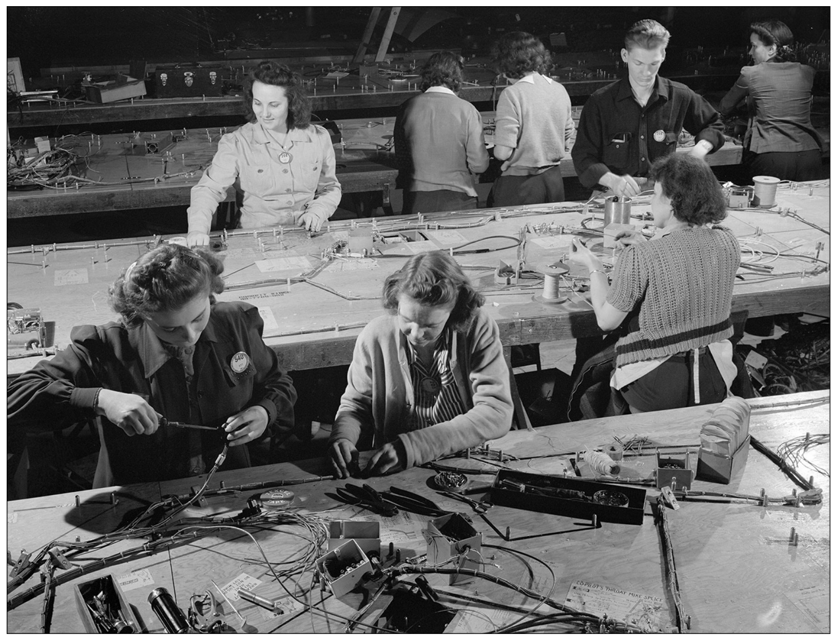
Women workers at a Boeing plant in Seattle assemble electrical components for the B-17 bomber. As men were recruited to the services, women came to play a vital part in American war production.
